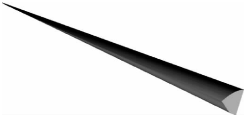
图 5 锥导乘波体外形 Fig. 5 Configuration of waverider derived from a conical flowfield
